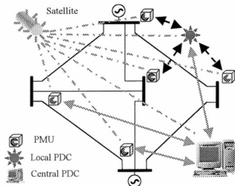
Fig. 1 – The structure of a monitoring system based on SPM (PMU – Phasor Measurement Unit, PDC – Phasor Data Concentrator).
