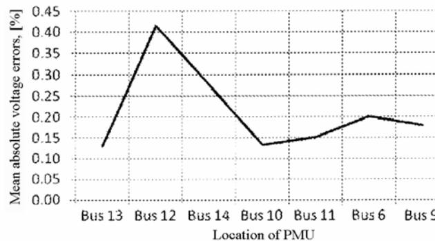
Fig. 3 – Average voltage errors in the IPS, for different levels of bus contingency and different location of 1 PMU.
