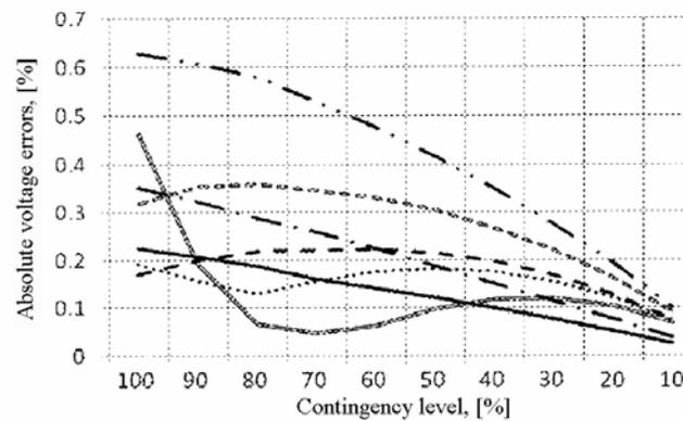
Fig. 2 – Voltage errors in the IPS, for different levels of bus contingency and different location of 1 PMU (for legend, see Table 2).
