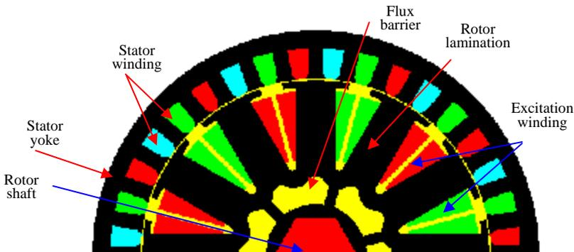
Fig. 2 – Cross section through the electromagnetic excitation semi-machine.
