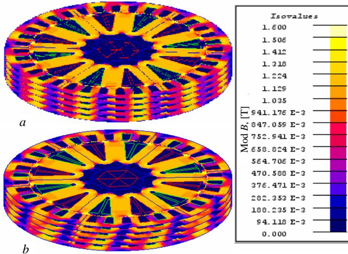
Fig. 4 – Flux density coloured map in the electromagnetic excitation semi-machine.
