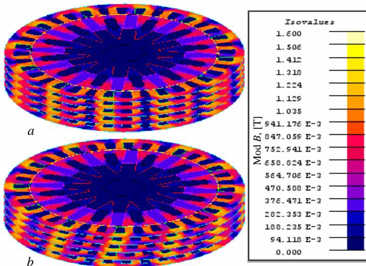
Fig. 3 – Flux density coloured map in the permanent magnet semi-machine.
