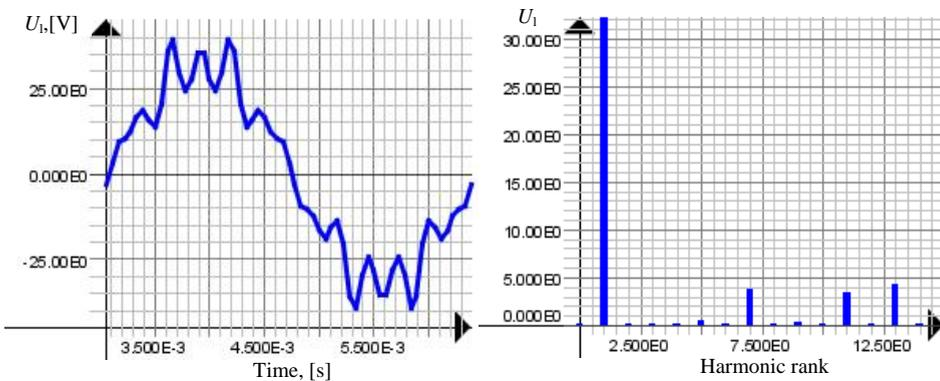
Fig. 7 – Line voltage and its decomposition into harmonics – initial situation.
