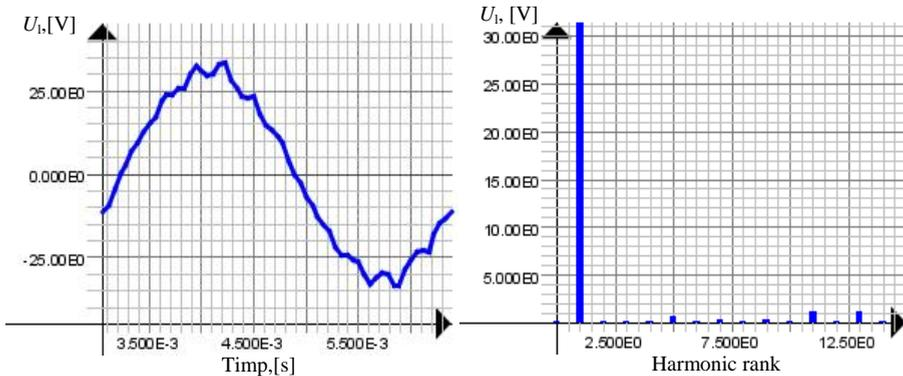
Fig. 8 – Line voltage and harmonics decomposition when the slot is 8 degrees skewed.
