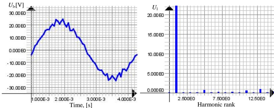
Fig. 6 – Line voltage and its decomposition into harmonics when the slot is 8 degrees.
