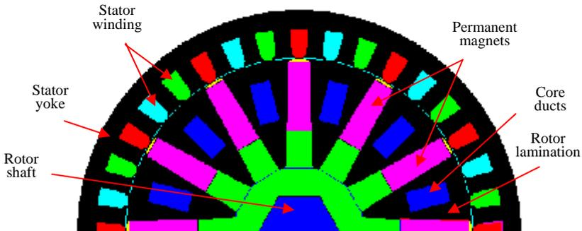
Fig. 1 – Cross section through the permanent magnet semi-machine.
