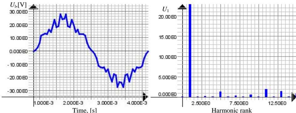
Fig. 5 – Line voltage and its decomposition into harmonics – initial situation.
