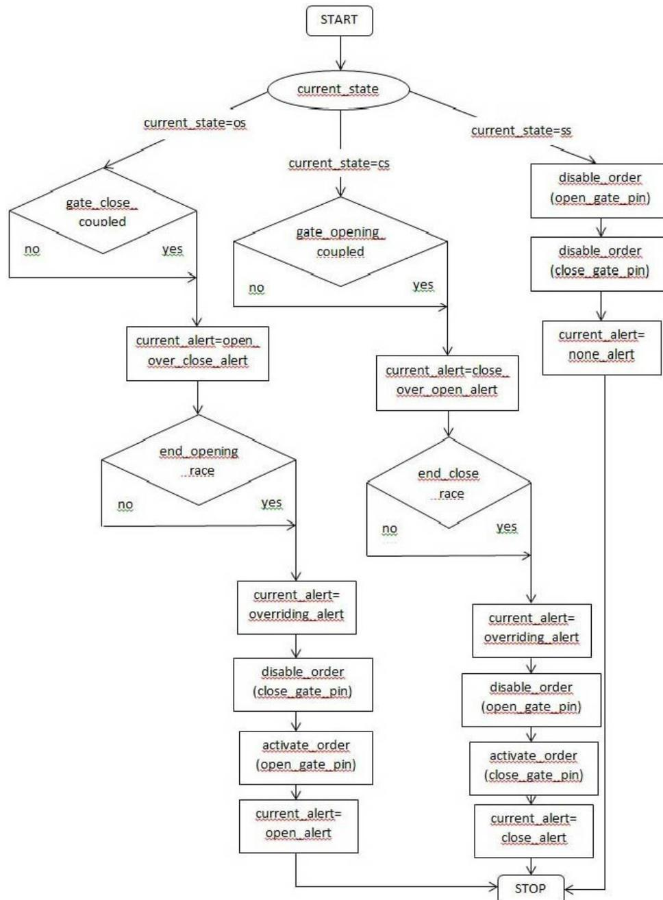
Fig. 3 – Flow chart illustrating the function of activation and deactivation of the order.
