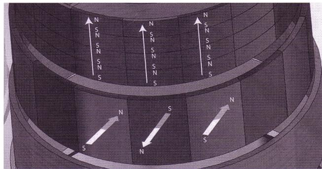
Fig. 6 – Alternating N-S poles radial magnets.
