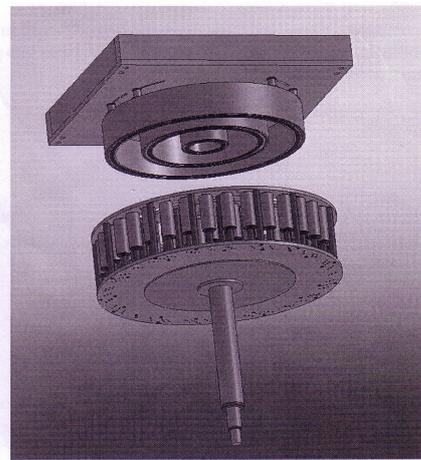
Fig. 5 – The static and rotating structures exploded view.
