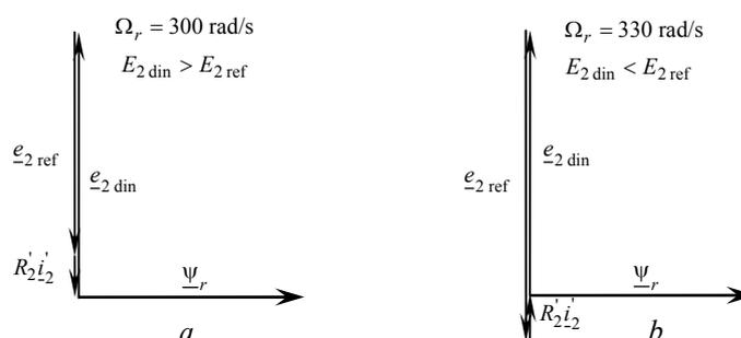
Fig. 3 – Rotor voltages phasors diagram in steady-state:
