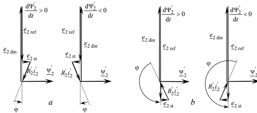
Fig. 6 – Rotor voltages phasors in transient: a – motor; b – generator.
