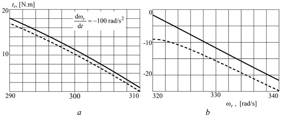
Fig. 12 – Comparing electromagnetic torques: *a* – motor; *b* – generator.
