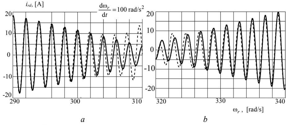
Fig. 10 – Comparing rotor currents: *a* – motor; *b* – generator.
