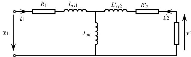
Fig. 2 – Simplified equivalent circuit.
