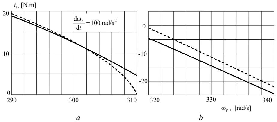
Fig. 11 – Comparing electromagnetic torques: *a* – motor; *b* – generator.
