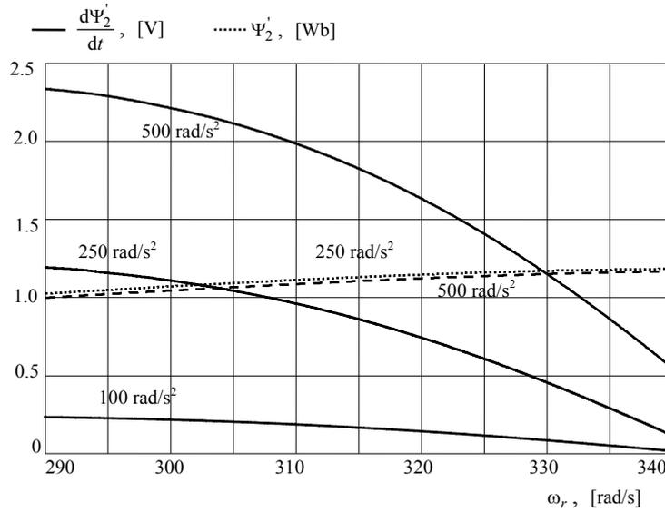
Fig. 5 – Rotor voltages phasors in transient vs. speed, for motor and generator working.
