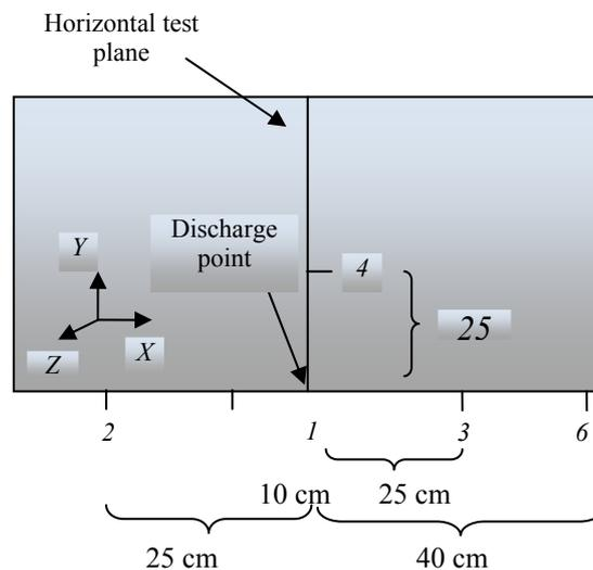
Fig. 1 – Measuring points on horizontal and vertical directions, on which magnetic field sensors are placed at different distances.
