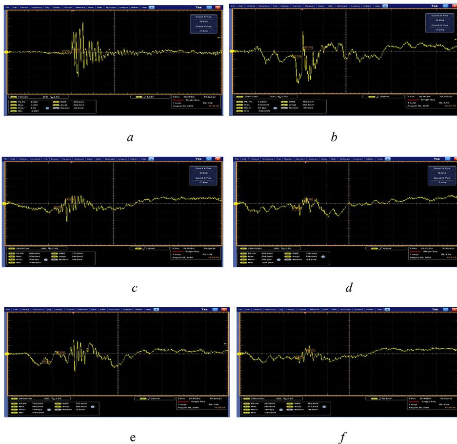
Fig. 5 – Waveforms of the magnetic field for + 2 kV charge (Z-axis).
