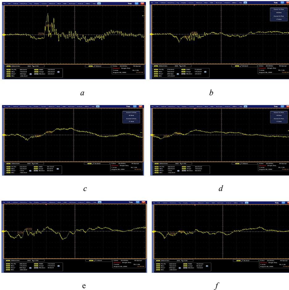
Fig. 3 – Waveforms of the magnetic field for +2 kV of charge ( $X$ -axis).
