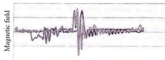
Fig. 7 – Magnetic field associated to the electrostatic discharges for all three directions orientation of the sensor, in point *I* of discharge.
