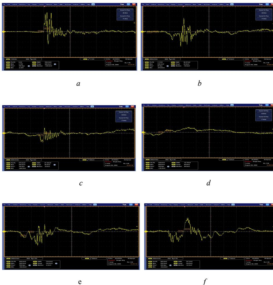
Fig. 4 – Waveforms of the magnetic field for + 2 kV charge (Y-axis).
