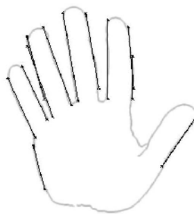
Fig. 2 –Straight lines detected on the hand contour.
