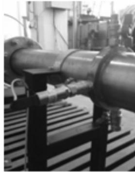
Fig. 5 – The pressure sensor mounted on the rig.
