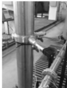
Fig. 6 – The outlet pressure sensor mounted on the rig.
