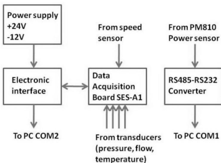
Fig. 4 –Data Acquisition System.
