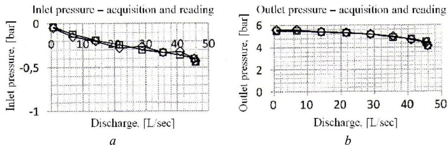
Fig. 9 – The inlet (a) and the outlet (b) pressures. □ curve – reading and ◇ curve – acquisition.
