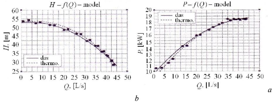
Fig. 11 – The head (a) and the mechanical power (b) vs. flow rate; the square-marked curves are obtained using the thermodynamic method (in both figures); the circle-marked curves are obtained with the rig's data acquisition system.
