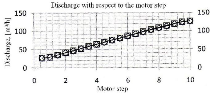
Fig. 10 – SITRANS and Krone flowmeters readings (□ for – SITRANS and ◇ for – Krone).
