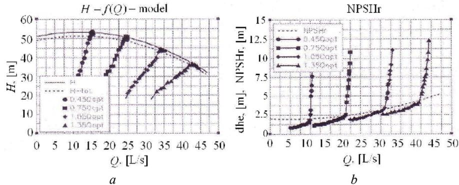
Fig. 12 – The head as a function of flow rate when functioning in cavitation (a) and the sensibility curve in cavitation (b).
