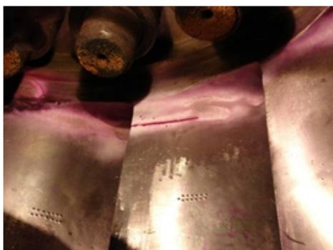
Fig. 1 – Fatigue crack in the runner blade.
