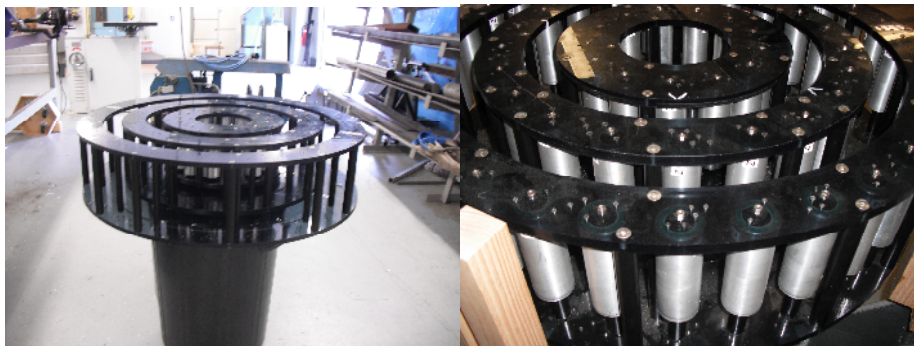
Fig. 13 – Concentric frames containing the cylinders.
