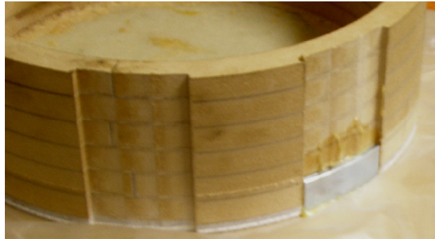
Fig. 5 – Grooves for magnets.
