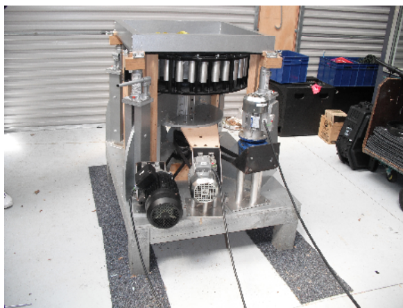
Fig. 15 – The three AC motors that rotate the frames.
