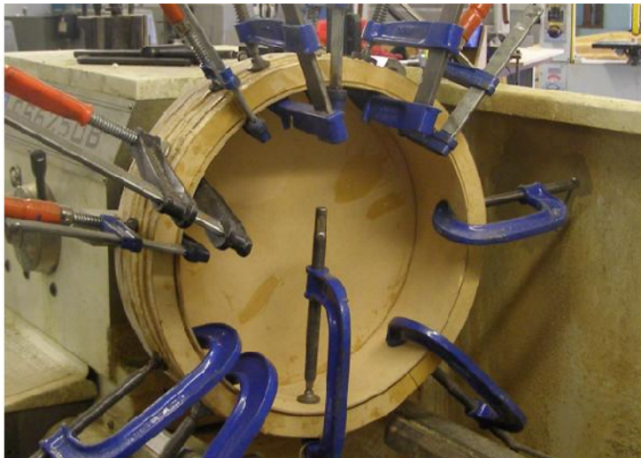
Fig. 11 – Clamping a thin wooden inner layer in place.
