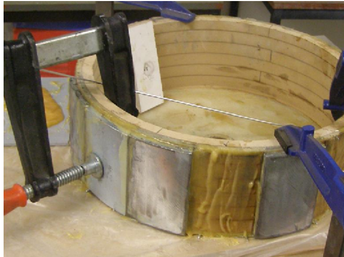
Fig. 10 – Clamping the radial magnets in place.
