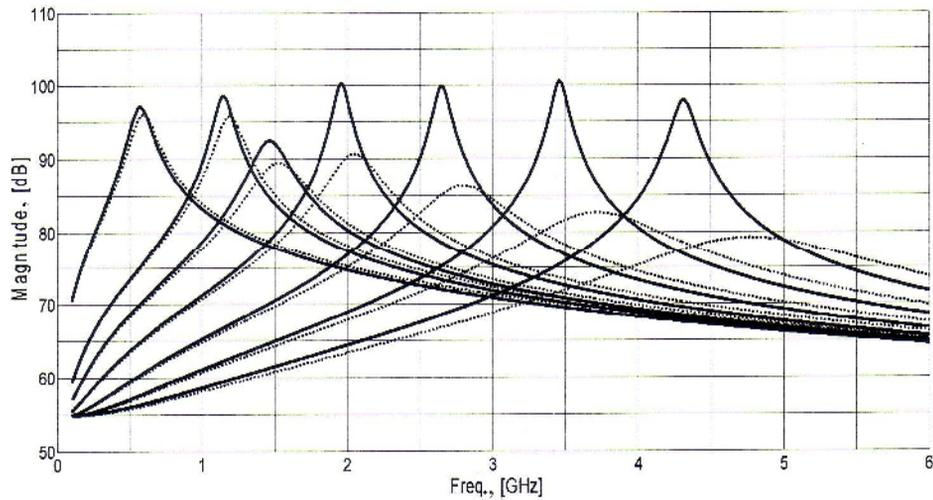
Fig. 4 – TOSI and *RLC* model frequency response for the first circuit.
