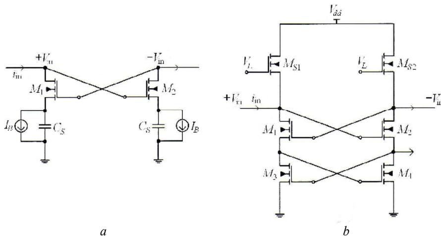
Fig. 2 – Differential active inductors.
