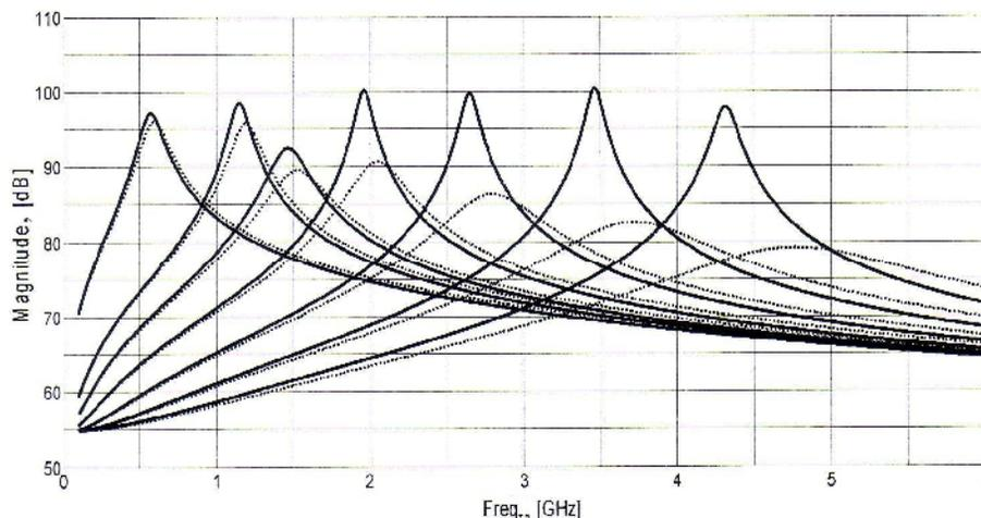
Fig. 5 – TOSI and  $RLC$  model frequency response for the second circuit.
