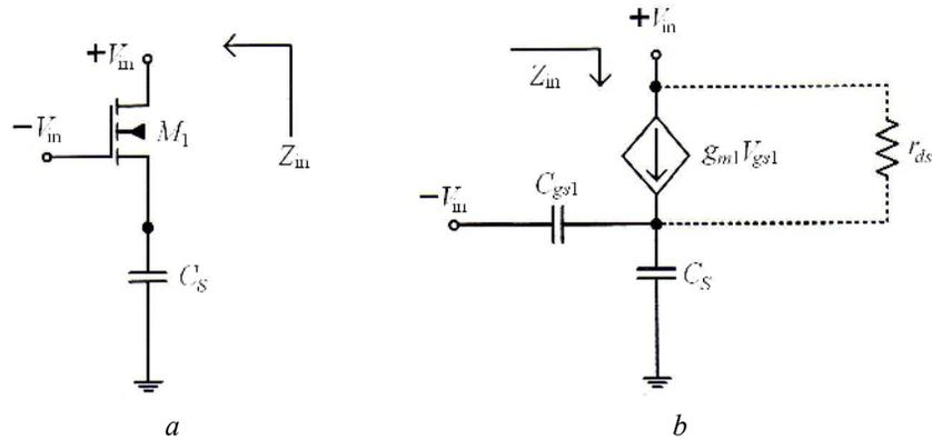
Fig. 1 – Single-ended active inductor (Ler *et al.*, 2008).
