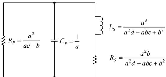
Fig. 4 – Equivalent *RLC* passive model proposed for TOSI.
