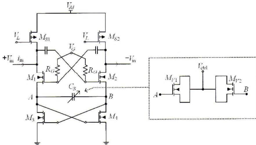
Fig. 3 – Differential active inductor with improved tuning capability and equivalent *RLC* passive model.
