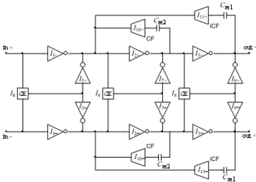
Fig. 6 – The ULV three-stage fully differential amplifier.
