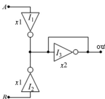
Fig. 5 – ULV inverting voltage averaging circuit.
