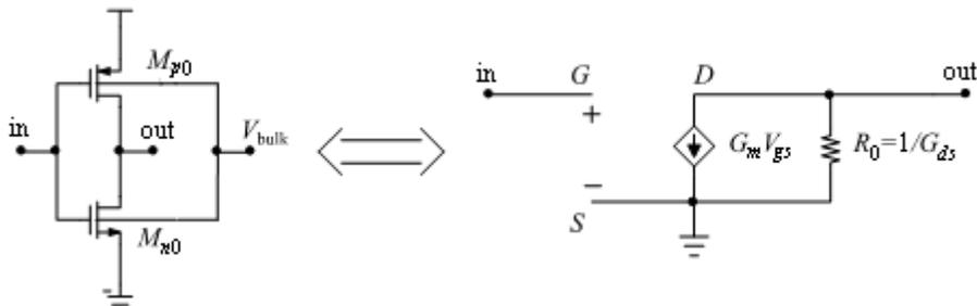
Fig. 1 – The ULV inverter and its small signal equivalent circuit.
