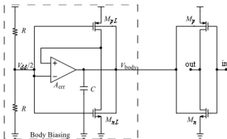
Fig. 2 – The body biasing circuit of an ULV inverter.
