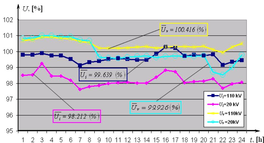
Fig. 6 – The voltage level variation, in percentages, during some working days from the cold winter and hot summer state from the analysed repartition system nodes: N03 – with 110 kV nominal voltage, N03-M20 – with 20 kV nominal voltage.
