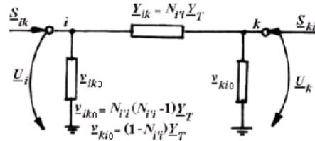
Fig. 3 – Equivalent four-pole for a power transformer with real transformation ratio ( $N_{iV}$ ).
