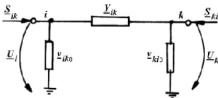
Fig. 2 – Equivalent four-pole for an overhead or cable power line.
