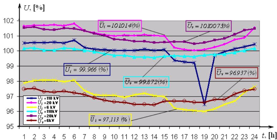
Fig. 5 – The voltage level variation, in percentages, during some working days from the cold winter and hot summer state from the analysed repartition system nodes: N13 – with 110 kV nominal voltage, N13-M20 – with 20 kV nominal voltage and N13-M6– with 6 kV nominal voltage.
