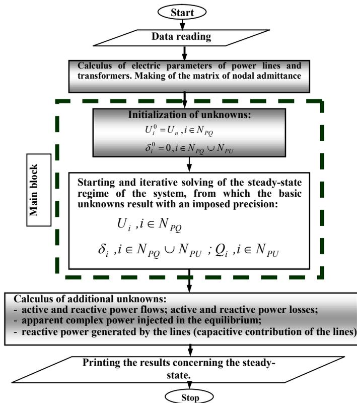
Fig. 1 – The steady-state computation diagram for an ERDS.
