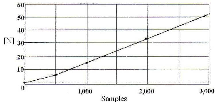
Fig. 3 – Force sensor characteristic for  $[0, \dots, 50 \text{ N}]$  range.
