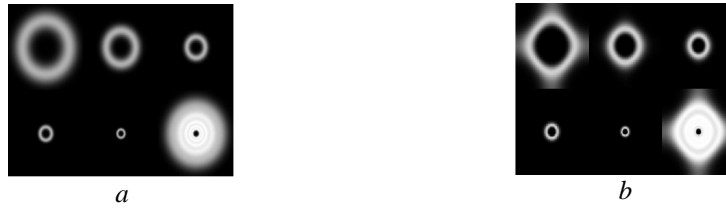
Fig. 5 – a – Circular ideal filter characteristics and their superposition; b – corresponding filter characteristics implemented with homogeneous CNN's.
