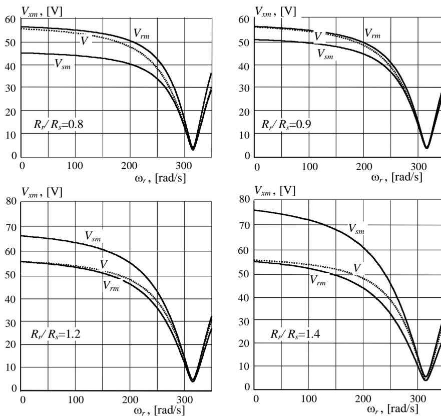
Fig. 5 – Voltage variations *versus* angular rotor speed.
