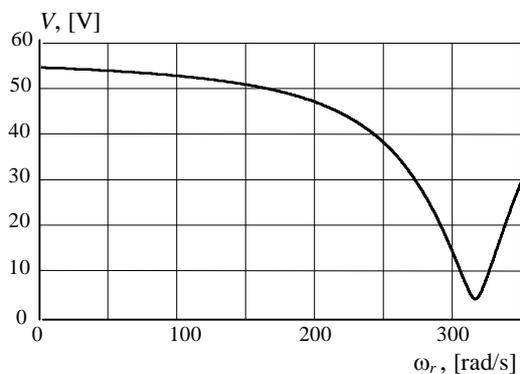
Fig. 4 – Voltage  $V$  variation *versus* angular rotor speed.
