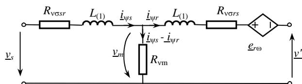
Fig. 6 – Simplified equivalent circuits of the two-phase model of the induction machine using fluxes.
