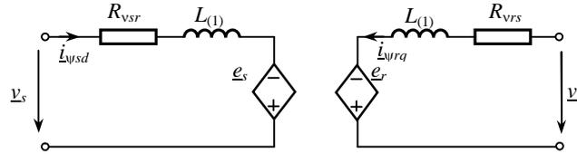
Fig. 1 – Equivalent circuits of the two-phase model of the induction machine in terms of fluxes.
