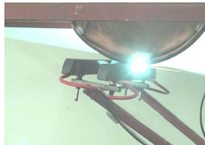
Fig. 3 – The electric arc between the rotating disc and the skates of a pantograph.
