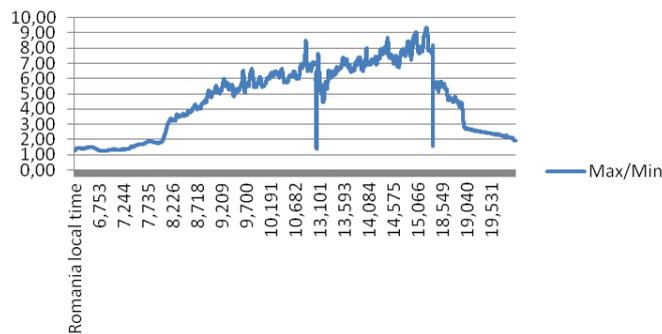
Fig. 7 – Ratio  $L_{max}/L_{min}$  between maximum and minimum illuminances.
