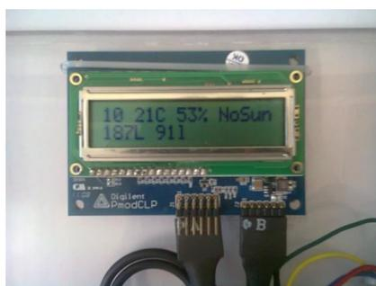
Fig. 4 –An example of data presented on the LCD display.
