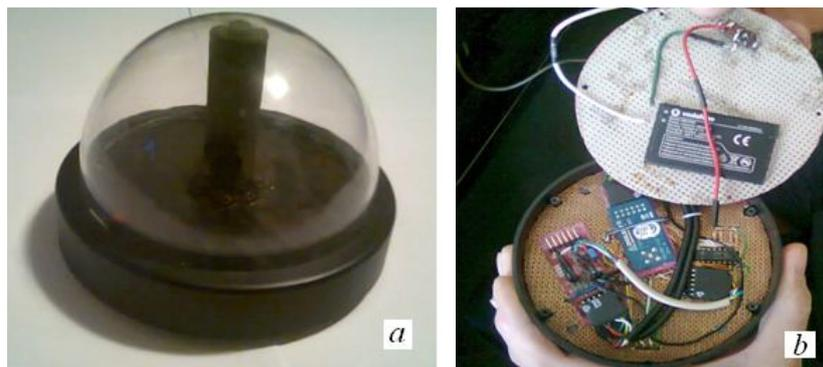
Fig. 3 – Sensor Module: *a* – front view; *b* – opened, back view.
