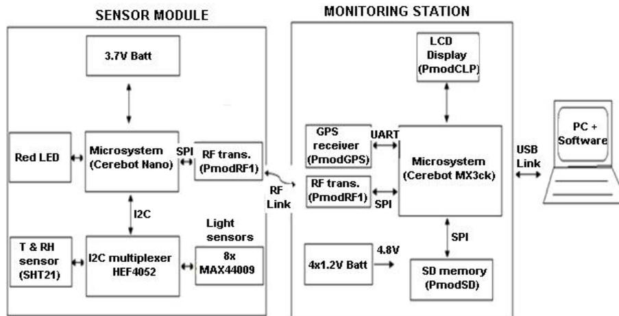
Fig.1 –Block diagram of the SD measurement system.
