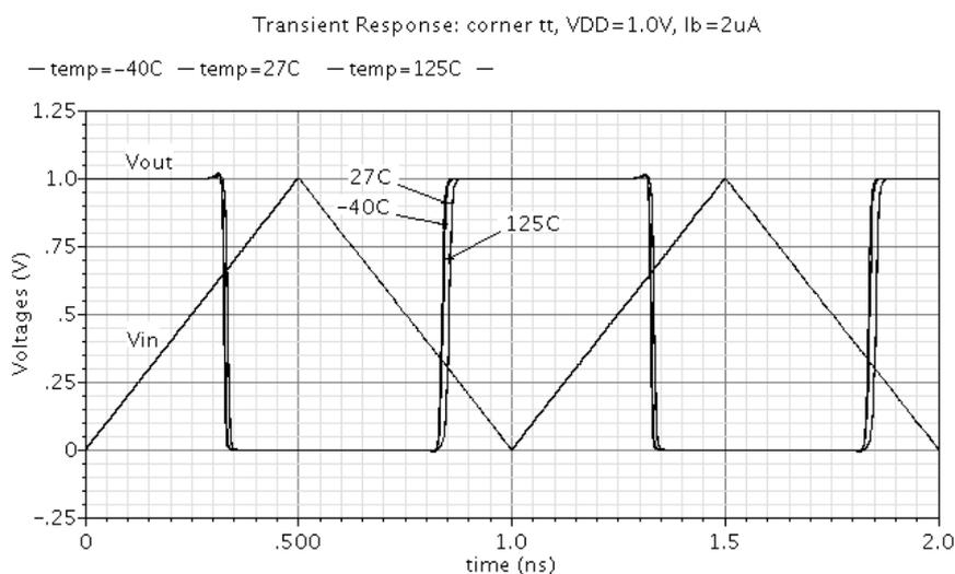
Fig. 8 – Switching thresholds versus temperature.
