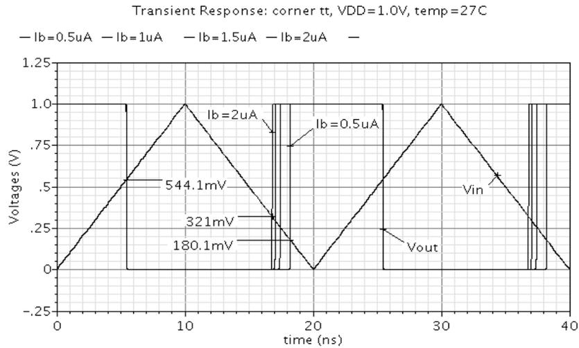
Fig. 4 – Transient responses to 50 MHz input signal.
