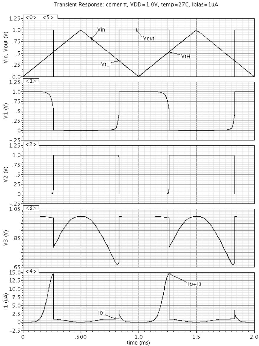
Fig. 3 – Waveforms specific to the proposed Schmitt trigger.
