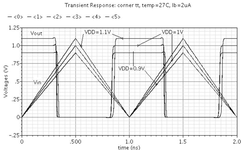
Fig. 7 – Switching thresholds versus supply voltage.
