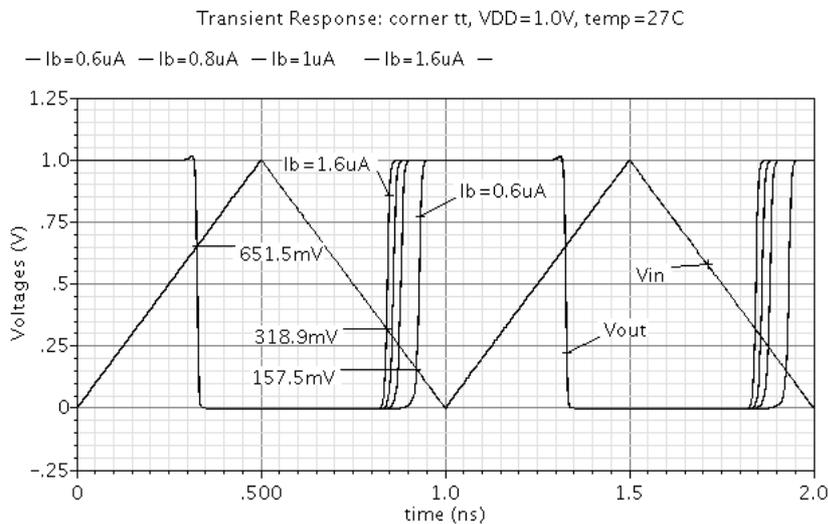
Fig. 5 – Transient responses to 1 GHz input signal.
