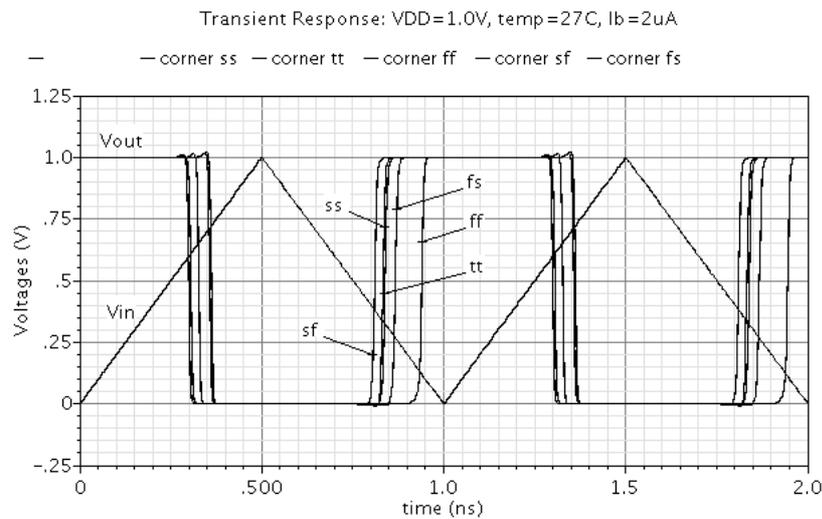
Fig. 6 – Switching thresholds versus process corners.
