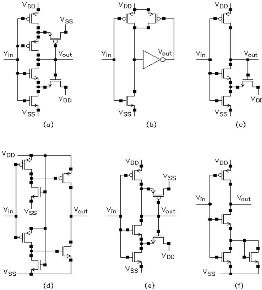
Fig. 1 – Configurations of CMOS Schmitt trigger circuits.
