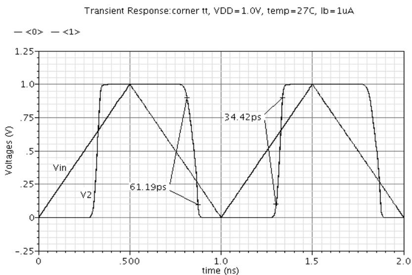
Fig. 9 – Rise and fall times corresponding to voltage  $V_2$ .
