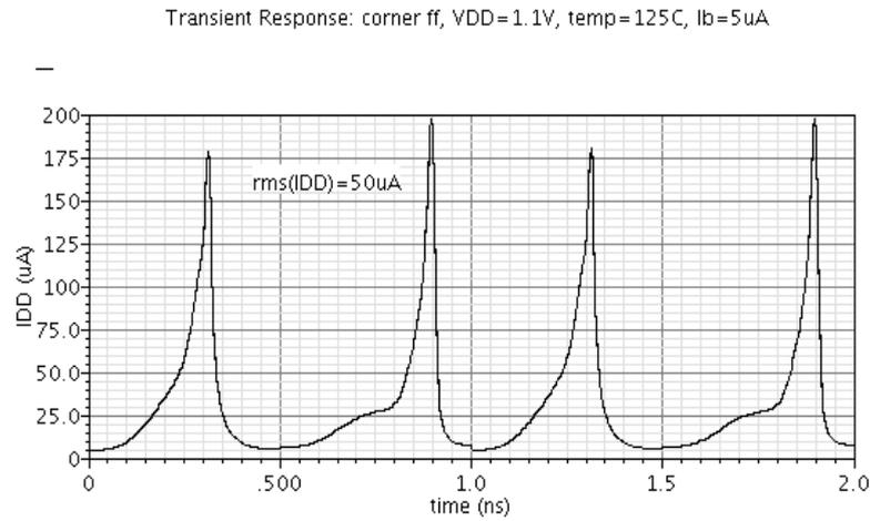
Fig. 10 – Supply current consumption.
