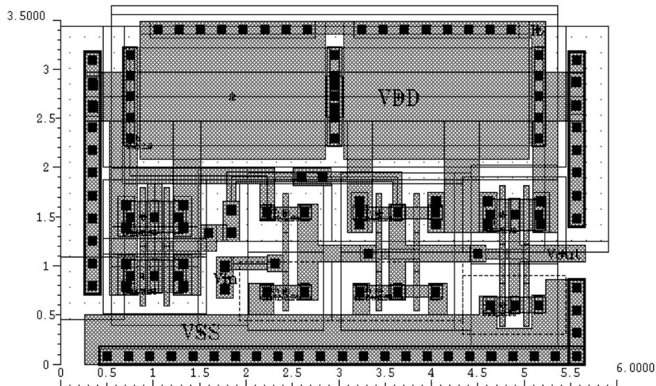
Fig. 11 – Layout view of the proposed Schmitt trigger.
