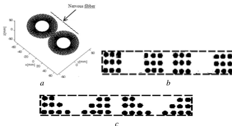
Fig. 2 – Distribution of turns inside the “eight” shape coil: *a* – commercial coil, disc shape, 9 turns/leaf in one plane; *b* – solenoid shape distributed on three layers (3 turns on each layer, for both leaves); *c* – solenoid shape distributed on three layers (4,3,2 turns on the three layers, for each leaf).
