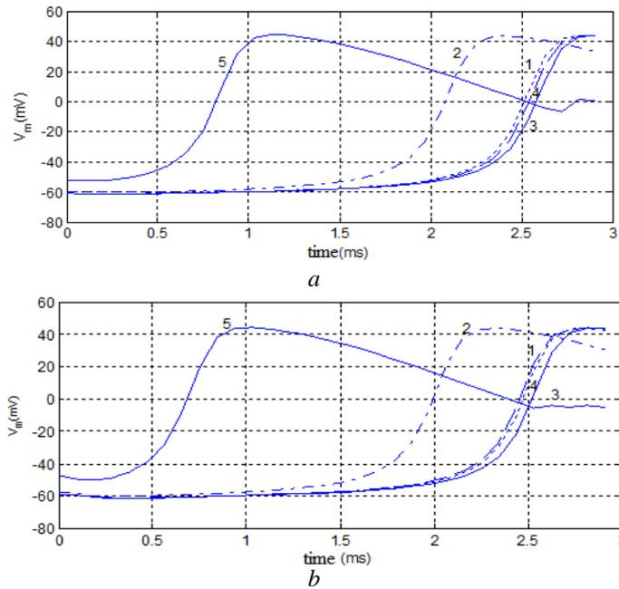
Fig. 3 – Time variation of the transmembrane potential, highlighting the latency period for each configuration: *a* – overdamped regime (for all the coils, the value of the circuit's capacitor is considered to be  $U_0 = 1,350$  V); *b* – underdamped regime (for all the coils, the value of the circuit's capacitor is considered to be  $U_0 = 1,600$  V).
