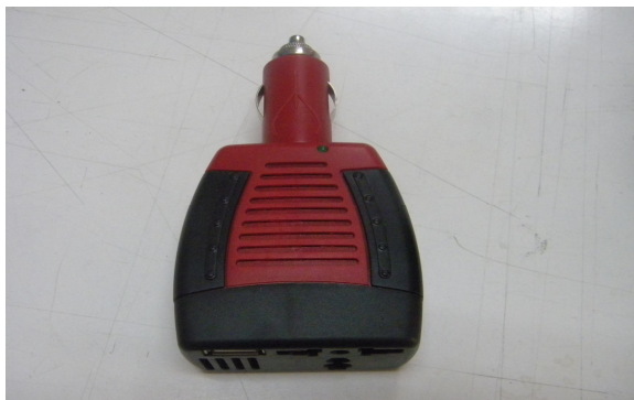
Fig. 6 – A commercial modified sine wave inverter.
