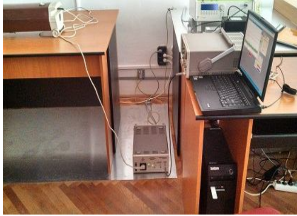
Fig. 4 – Testing stand for electromagnetic disturbances produced through conduction in the supply line from the Electromagnetic Compatibility Laboratory of Cluj Napoca Technical University.
