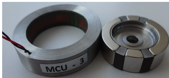
Fig. 6 – The experimental model of DC-TM.
