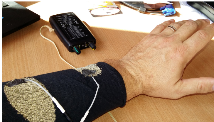
Fig. 6 – Knitted electrodes within a functional textile to produce the required functional electrical stimulation.
