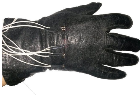
Fig. 5 – Glove with sensors for copying the healthy hand movements.
