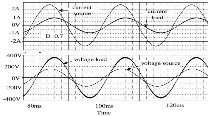
Fig. 5 – Waveforms of the  $i_m$  current,  $i_0$  current and  $v_m$  voltage,  $v_0$  voltage for  $D = 0.7$ , in the resistive load case  $R = 150 \Omega$ .
