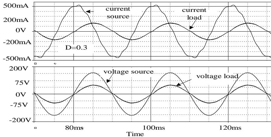
Fig. 3 – Waveforms of the  $i_m$  current,  $i_0$  current and  $v_m$  voltage,  $v_0$  voltage for  $D = 0.3$ , in the resistive load case  $R = 150 \Omega$ .
