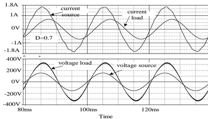
Fig. 6 – Waveforms of the  $i_m$  current,  $i_0$  current and  $v_m$  voltage,  $v_0$  voltage for  $D = 0.7$ , in the inductive load case ( $L = 750$  mH and  $R = 150 \Omega$ ).
