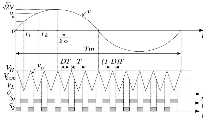
Fig. 2 – The waveform of the  $v$  voltage and the generation of the control signal for IGBT's.
