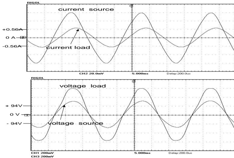
Fig. 11. Waveforms of the  $i_m$  current,  $i_o$  current and  $v_m$  voltage,  $v_o$  voltage for  $D = 0.7$ , in the inductive load case ( $L = 750 \text{ mH}$  and  $R = 150 \Omega$ ).
