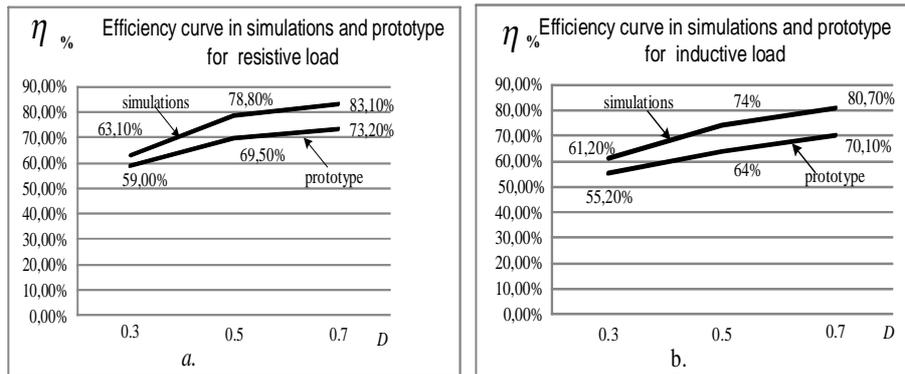
Fig. 13 – Efficiency: *a* – for the resistive load, *b* – for the inductive load.
