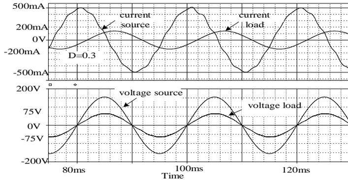
Fig. 4 – Waveforms of the  $i_m$  current,  $i_0$  current and  $v_m$  voltage,  $v_0$  voltage for  $D = 0.3$ , in the inductive load case ( $L = 750$  mH and  $R = 150 \Omega$ ).
