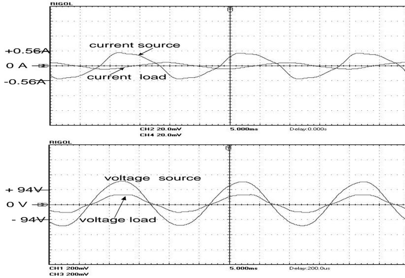
Fig. 9 – Waveforms of the  $i_m$  current,  $i_0$  current and  $v_m$  voltage,  $v_0$  voltage for  $D = 0.3$ , in the inductive load case ( $L = 750 \text{ mH}$  and  $R = 150 \Omega$ ).
