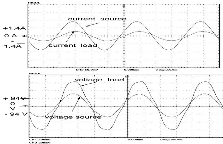
Fig. 10 – Waveforms of the  $i_m$  current,  $i_0$  current and  $v_m$  voltage,  $v_0$  voltage for  $D = 0.7$ , in the resistive load case  $R = 150 \Omega$ .
