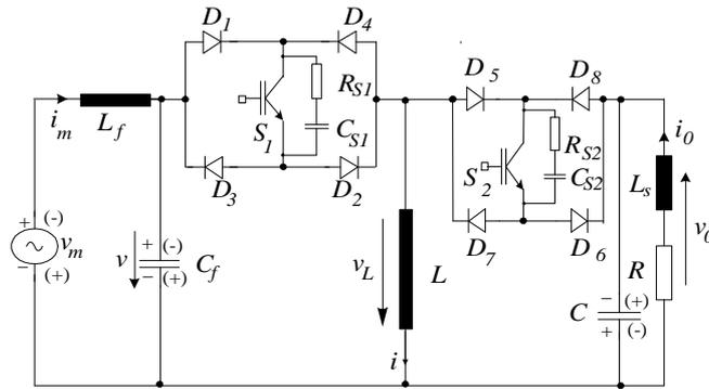
Fig. 1 – Single-phase direct ac-ac buck-boost converter.
