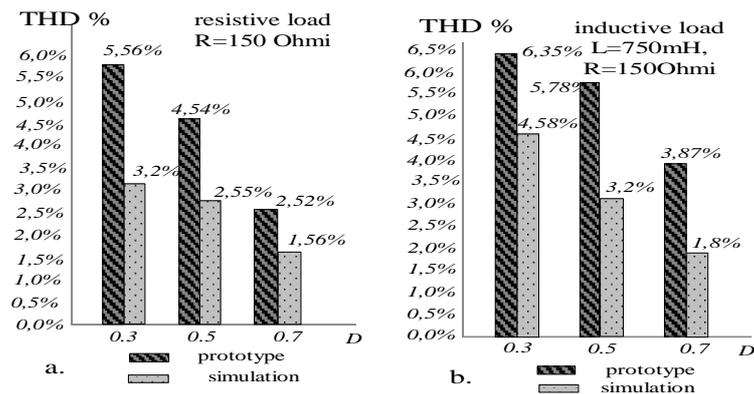
Fig. 12 – THD analysis for the input current: *a* – for the resistive load, *b* – for inductive load.
