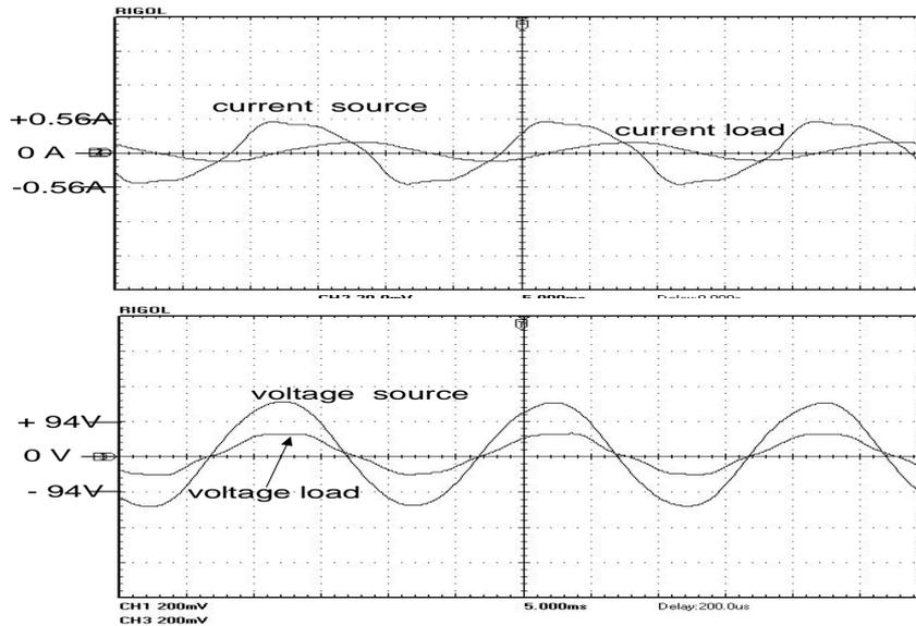
Fig. 8 – Waveforms of the  $i_m$  current,  $i_0$  current and  $v_m$  voltage,  $v_0$  voltage for  $D = 0.3$ , in the resistive load case  $R = 150 \Omega$ .
