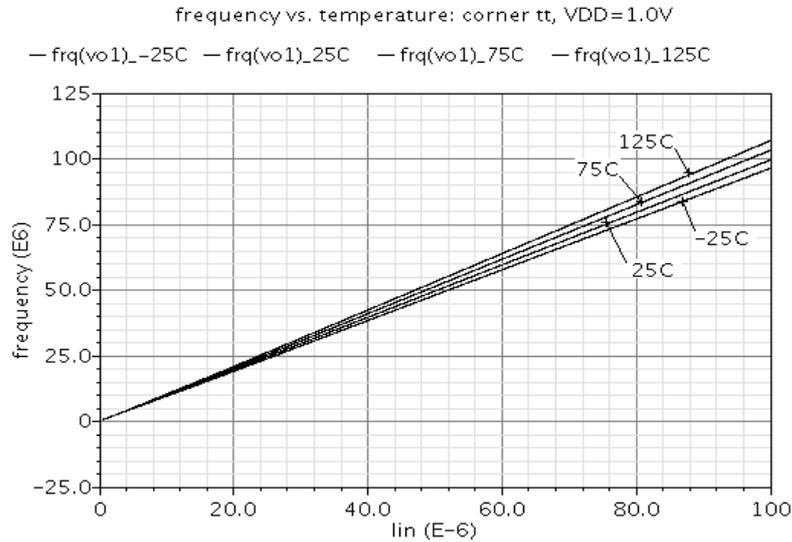
Fig. 7 – Influence of temperature on transfer characteristic.
