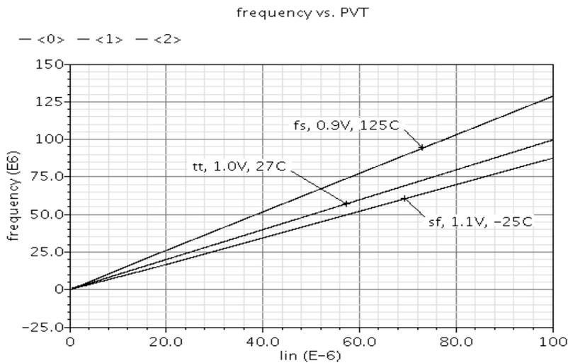
Fig. 8 – Influence of temperature on transfer characteristic.
