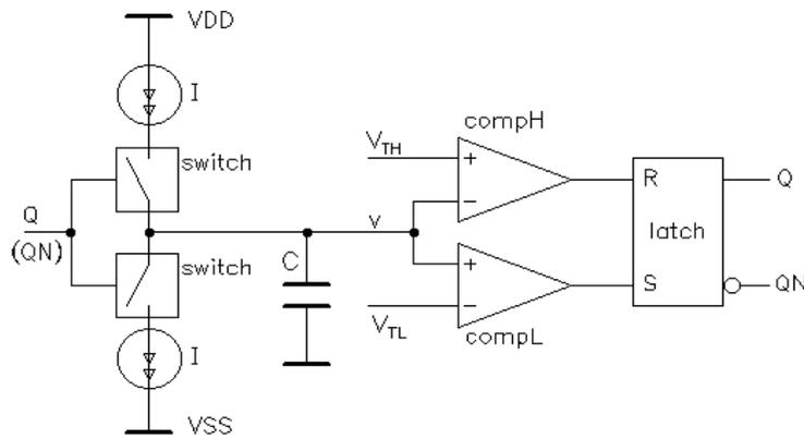
Fig. 1 – Generic current-to-frequency conversion principle.
