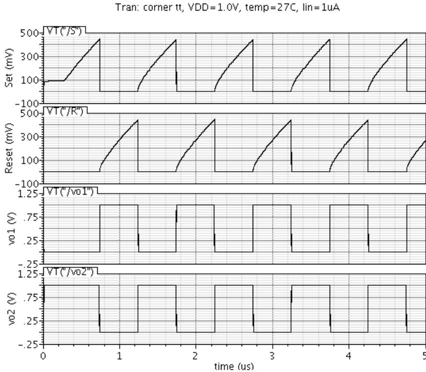
Fig. 3 – Transient responses of the circuit in Fig. 2.
