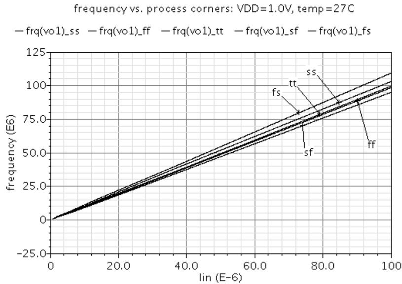
Fig. 5 – Influence of process corners on transfer characteristic.
