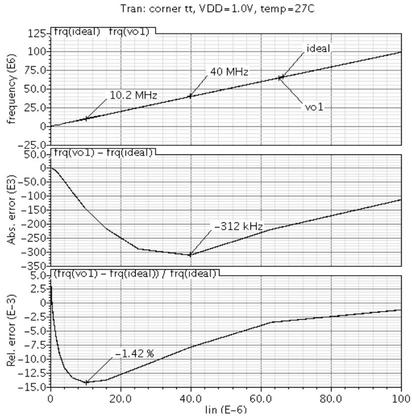
Fig. 4 – Transfer characteristic and linearity errors.
