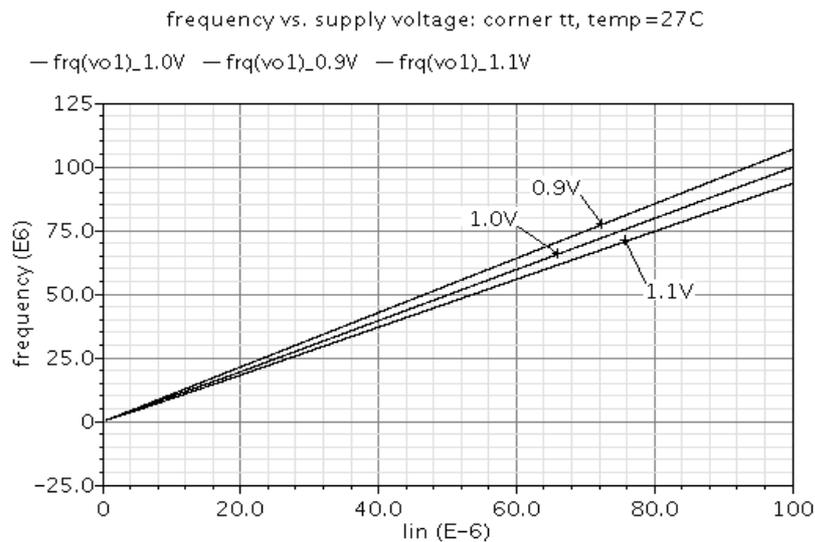
Fig. 6 – Influence of supply voltage on transfer characteristic.
