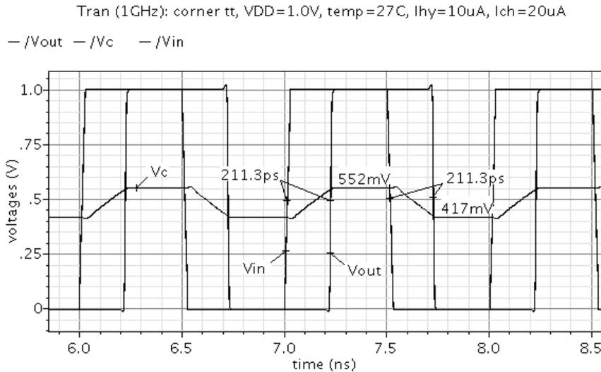
Fig. 6 – Delaying a signal of 1 GHz frequency.
