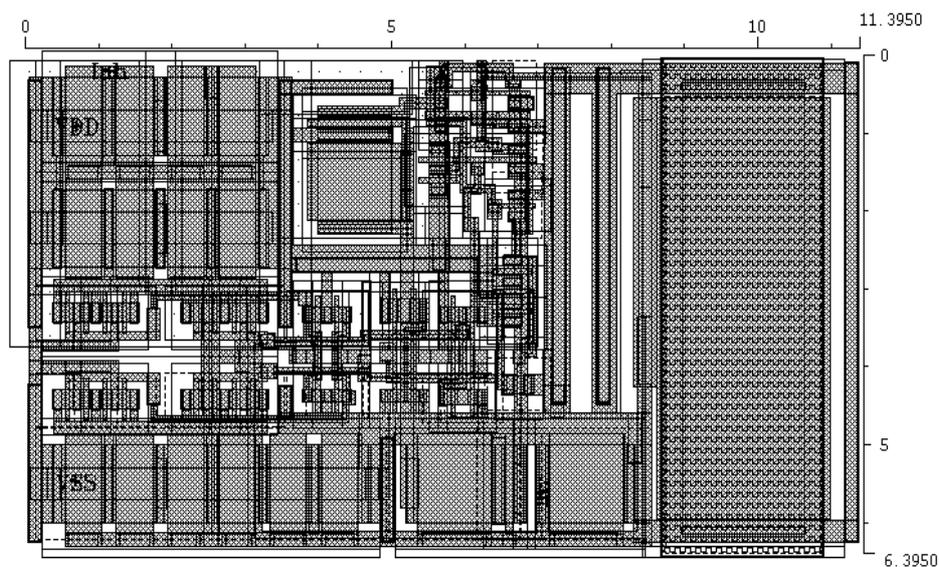
Fig. 11 – Layout of the proposed delay cell.
