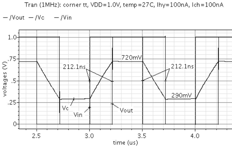
Fig. 4 – Delaying a signal of 1 MHz frequency.
