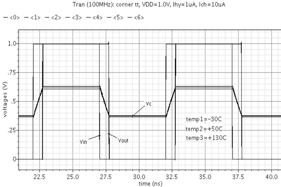
Fig. 7 – Influence of temperature on the delay.
