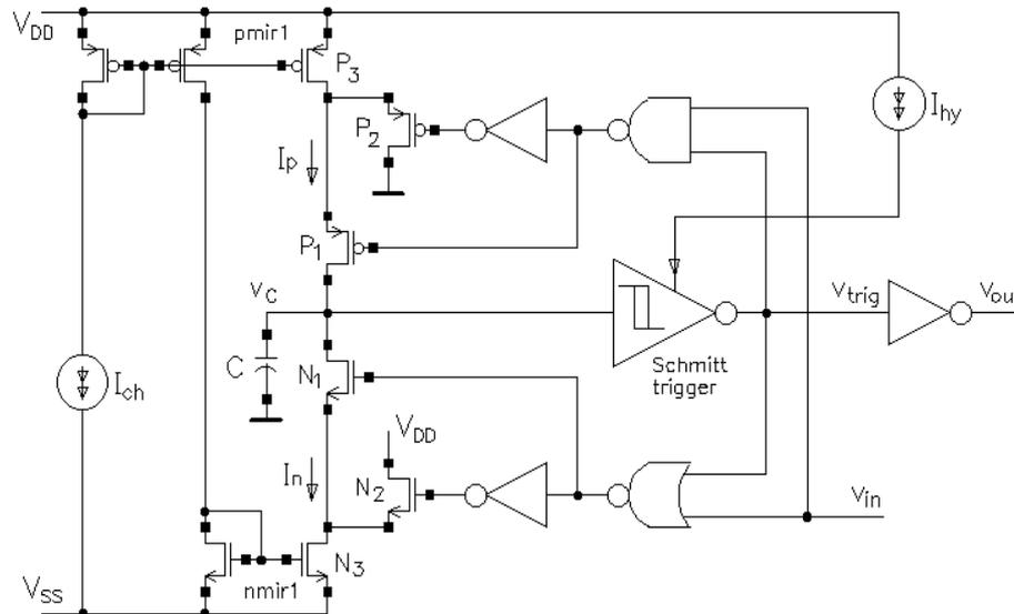
Fig. 2 – Schematic of the proposed delay cell.
