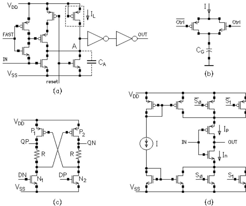
Fig. 1 – CMOS delay cells.
