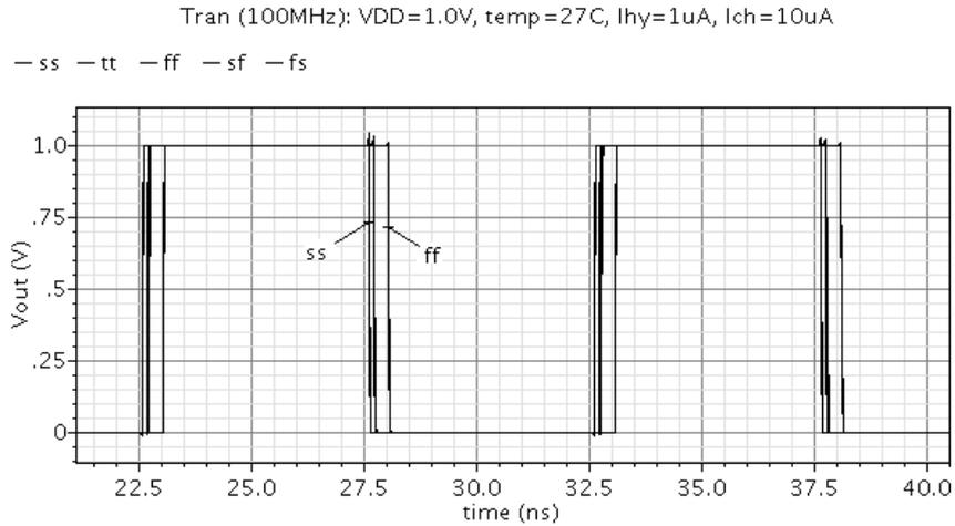
Fig. 9 – Influence of process corners on the delay.
