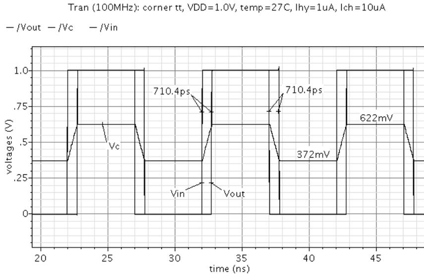
Fig. 5 – Delaying a signal of 100 MHz frequency.
