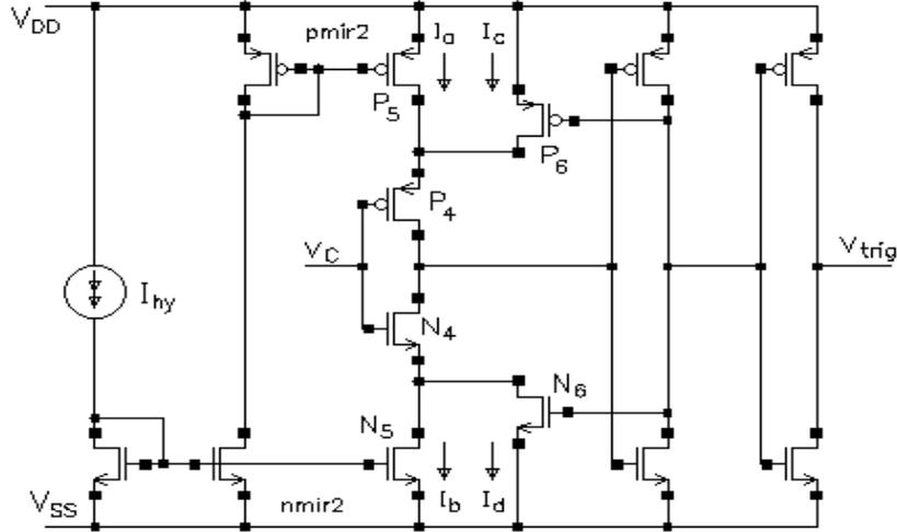
Fig. 3 – Schematic of the Schmitt trigger.
