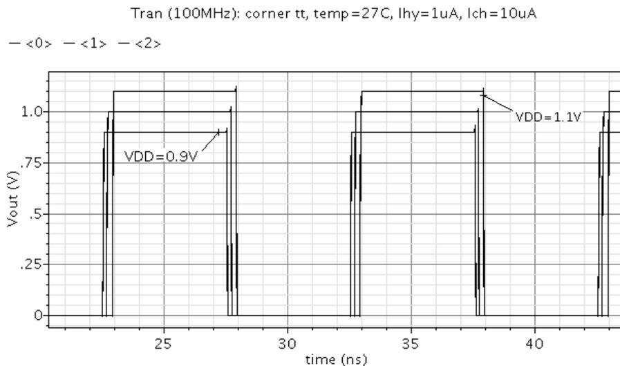
Fig. 8 – Influence of supply voltage on the delay.
