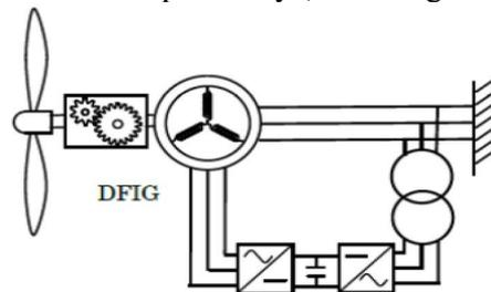
Fig. 1 – DFIG wind turbine model.
