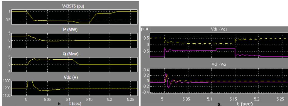
Fig. 5 – DC-link voltage, Active and Reactive power, Stator and Rotor voltage, for two-phase-to-ground fault.
