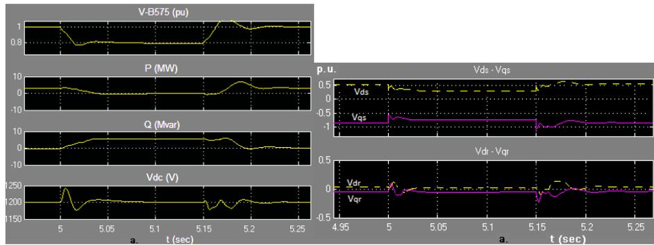
Fig. 4 – DC-link voltage, Active and Reactive power, Stator and Rotor voltage, for single-phase-to-ground grid fault.
