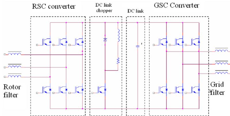
Fig. 2 – DFIG wind turbine power converter.
