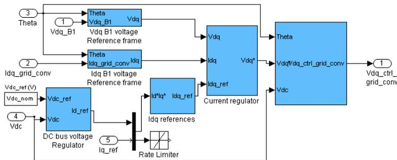
Fig. 3 – Simulink GSC converter control diagram.
