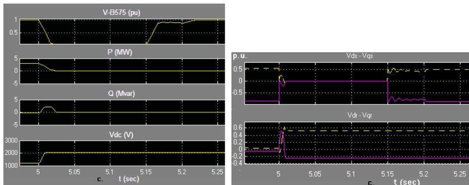
Fig. 6 – DC-link voltage, Active and Reactive power, Stator and Rotor voltage, for three phase grid fault.
