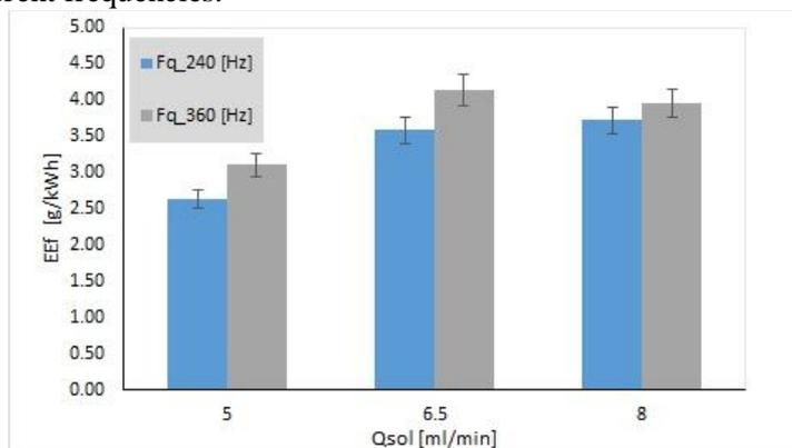
Fig. 11 – The evolution of the H<sub>2</sub>O<sub>2</sub> efficiency production yield for different water flow rates and different frequencies in SDR reactors assembly- three reactors.
