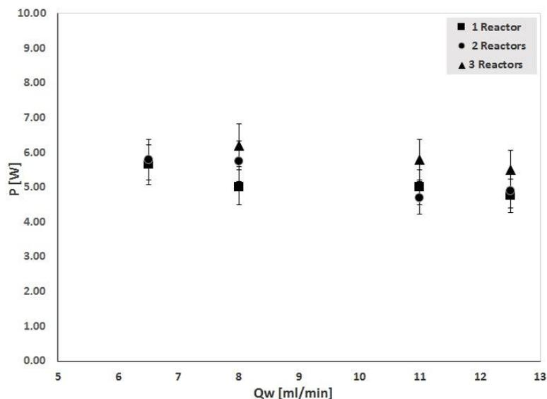
Fig. 8 – The evolution of the power for different water flow rates in SDR reactors assembly.
