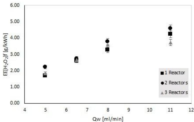
Fig. 9 – The evolution of the H<sub>2</sub>O<sub>2</sub> efficiency production yield for different water flow rates in SDR reactors assembly.
