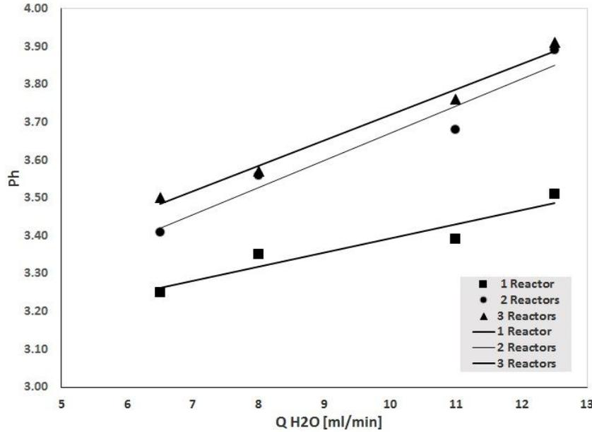
Fig.7 – The evolution of the pH in SDR reactors assembly.
