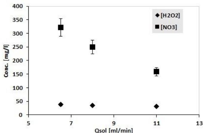
Fig. 5 – Reactive species concentrations level for one reactor SDR configuration with water flow rate for air as working gas.
