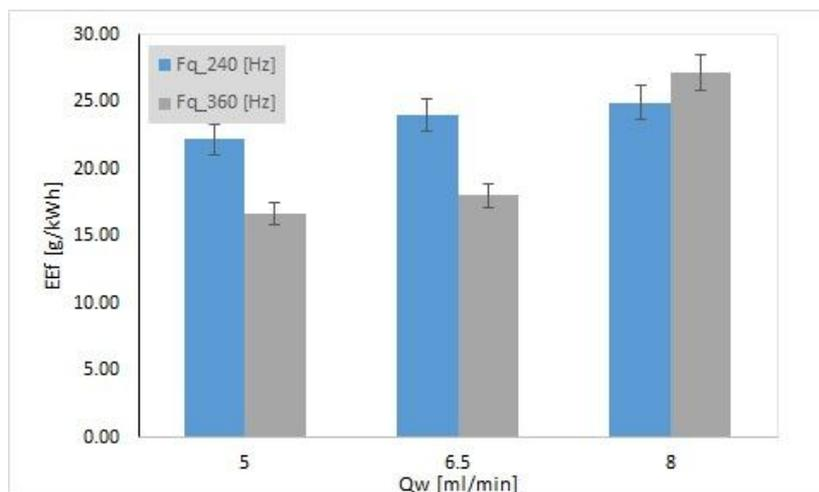
Fig. 12 – The evolution of the H<sub>2</sub>O<sub>2</sub> efficiency production yield for different water flow rates, and different frequencies in SDR reactors assembly – three reactors configuration.
