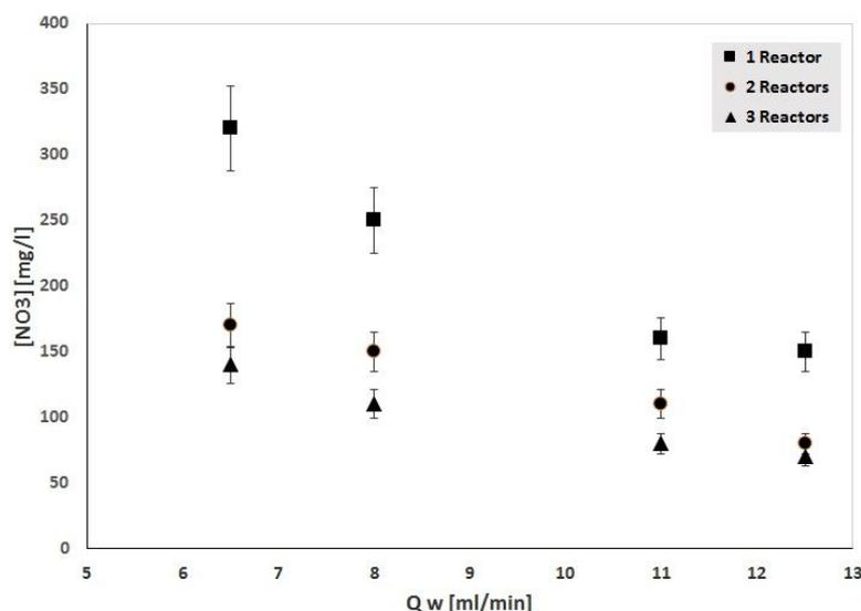
Fig. 4 – The evolution of the  $\text{NO}_3$  concentration produced in water in the SDR reactors with water flow rate for air as working gas.
