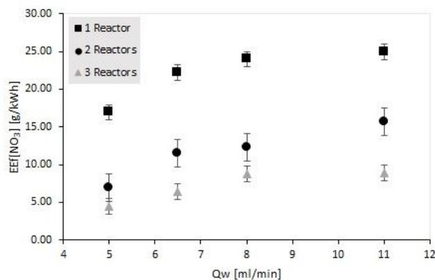
Fig. 10 – The evolution of the NO<sub>3</sub> efficiency production yield for different water flow rates in SDR reactors assembly.
