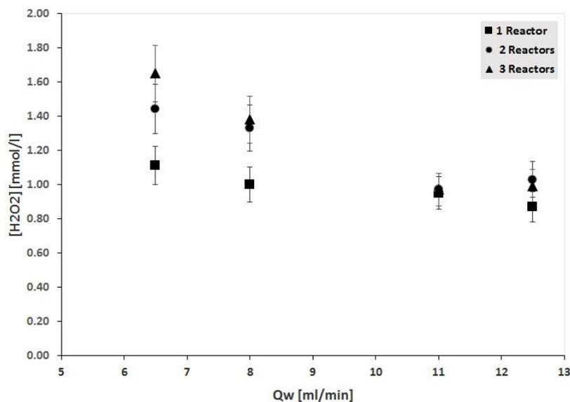
Fig. 3 – The evolution of the hydrogen peroxide concentration produced in water in the SDR reactors with air as working gas.
