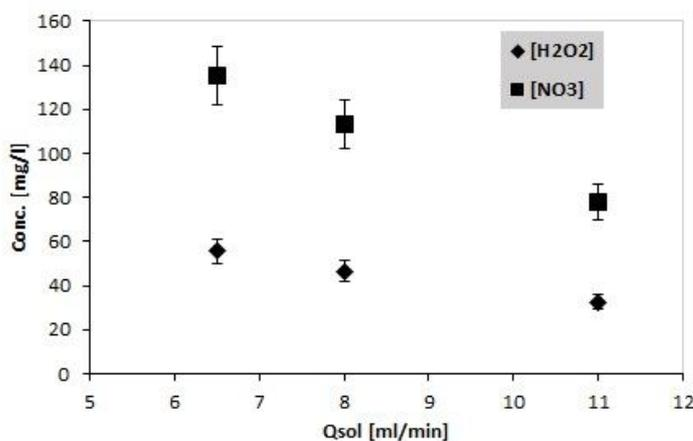
Fig. 6 – Reactive species concentrations level for three reactor SDR configuration with water flow rate for air as working gas.
