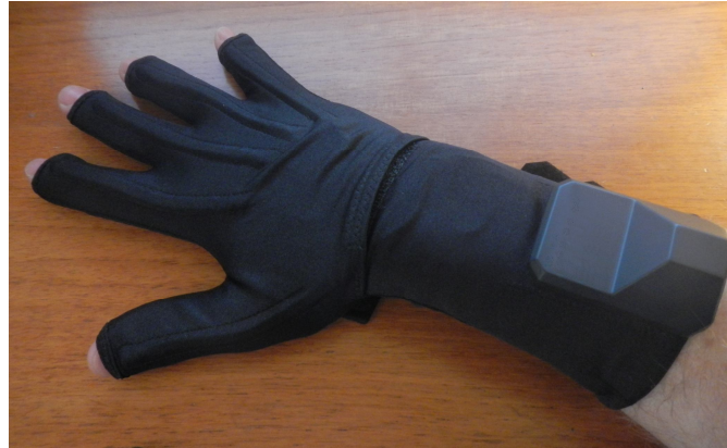
Fig. 3 – Data glove – equipped with bending sensor on each finger.
