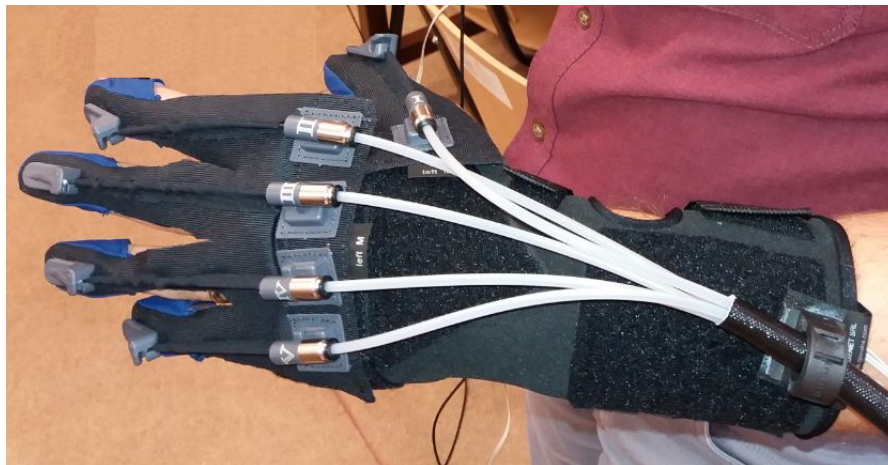
Fig. 1 – Overview of the robotic glove with metal tendons attached.
