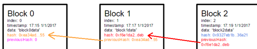
Fig. 1 – Simple Blockchain structure.
