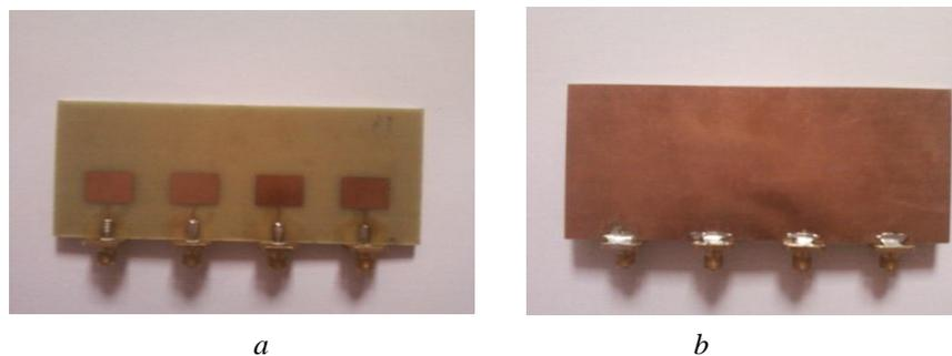
Fig. 9 – Photograph of setup of fabricated CMAA for mutual coupling measurement.
