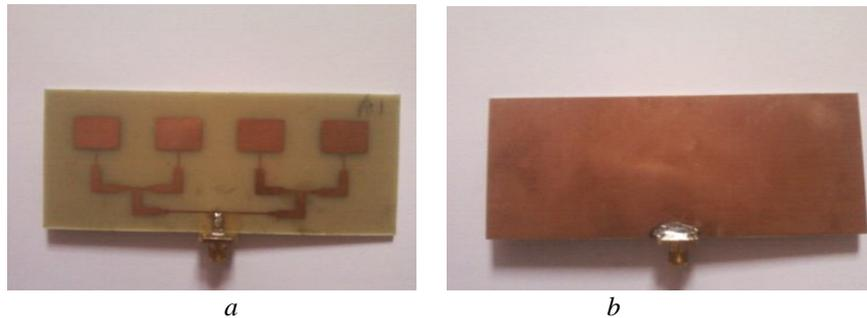
Fig. 8 – Photograph of fabricated CMAA.
