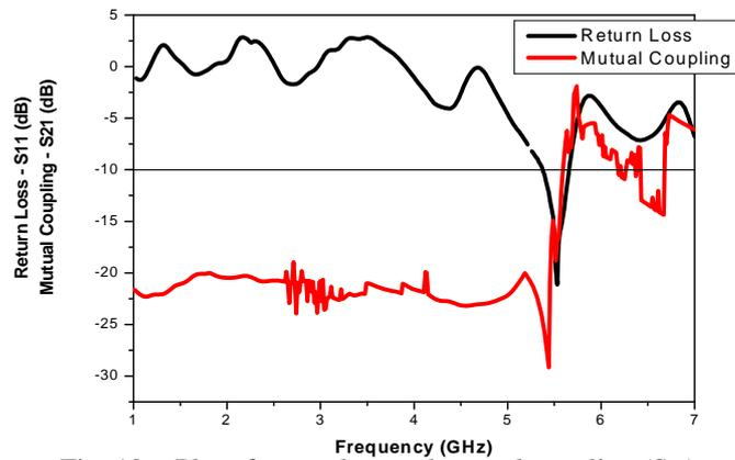
Fig. 12 – Plot of return loss and mutual coupling ( $S_{21}$ ) versus frequency of CMAA.
