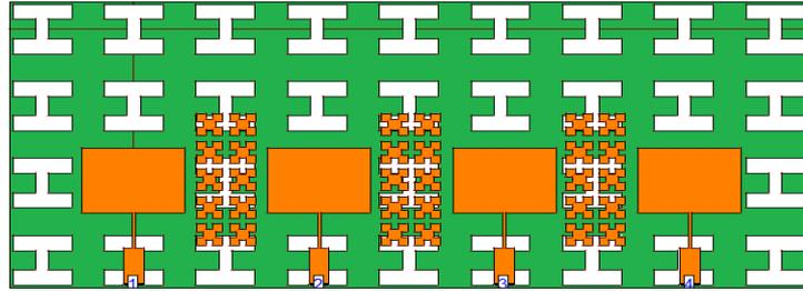
Fig. 7 – Schematic of setup of proposed microstrip antenna array for mutual coupling measurement.
