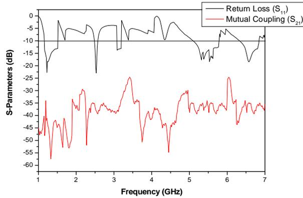
Fig. 16 – Plot of return loss and mutual coupling ( $S_{21}$ ) versus frequency of proposed microstrip antenna array.
