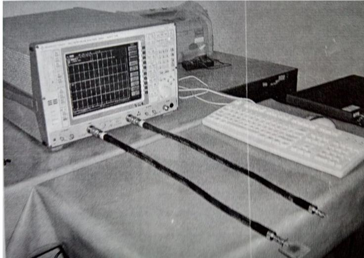
Fig. 15 – Photograph of experimental setup to measure return loss and mutual coupling.
