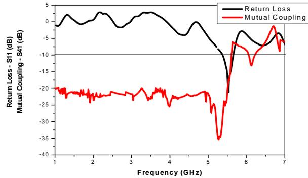
Fig. 14 – Plot of return loss and mutual coupling ( $S_{41}$ ) versus frequency of CMAA.
