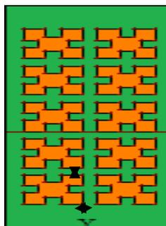
Fig. 5 – Schematic of fractal shape patch EBG structure.
