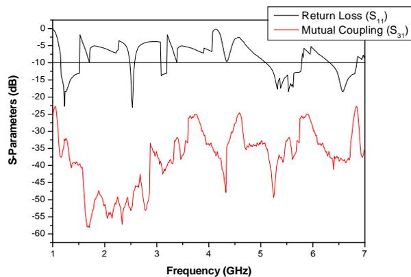
Fig. 17 – Plot of return loss and mutual coupling ( $S_{31}$ ) versus frequency of proposed microstrip antenna array.
