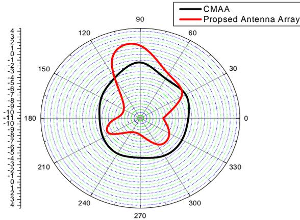
Fig. 19 – Plots of radiation patterns of CMAA and proposed microstrip antenna array.
