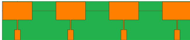
Fig. 2 – Schematic of setup of CMAA for mutual coupling measurement.
