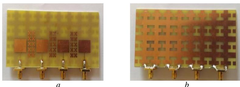
Fig. 11 – Photograph of setup of fabricated proposed microstrip antenna array for mutual coupling measurement.
