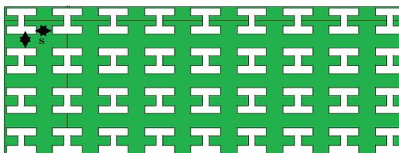
Fig. 4 – Schematic of I shape slot EBG structure.
