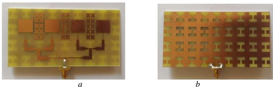
Fig. 10 – Photograph of fabricated proposed microstrip antenna array.
