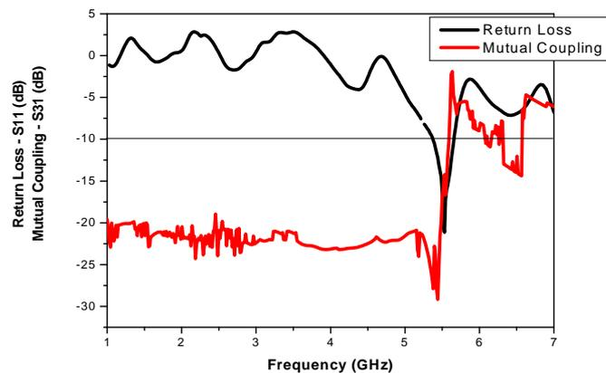
Fig. 13 – Plot of return loss and mutual coupling ( $S_{31}$ ) versus frequency of CMAA.
