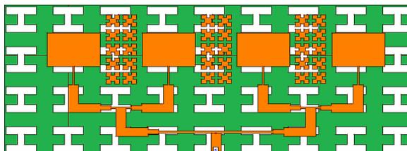
Fig. 6 – Schematic of proposed microstrip antenna array.
