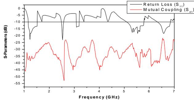
Fig. 18 – Plot of return loss and mutual coupling ( $S_{41}$ ) versus frequency of proposed microstrip antenna array.
