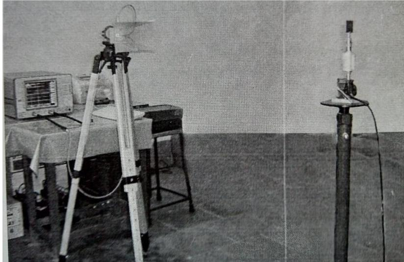
Fig. 20 – Photograph of experimental setup to measure radiation pattern.
