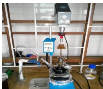
Fig. 1 – Experimental setup for synthesis of Fe 3 O 4
