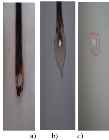
Fig. 4 – Samples of studied materials after the test of fire behaviour a) Compact polycarbonate, b) PPs, c) PMMA Plazcast.
