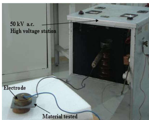
Fig. 6 – The experimental equipment used for the dielectric rigidity.
