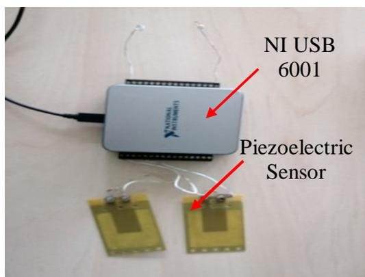
Fig. 2 – Sensors to the acquisition board.
