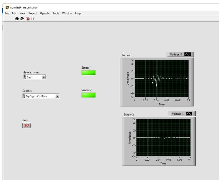
Fig. 3 – The front panel of the virtual instrument for the case „Light on”.
