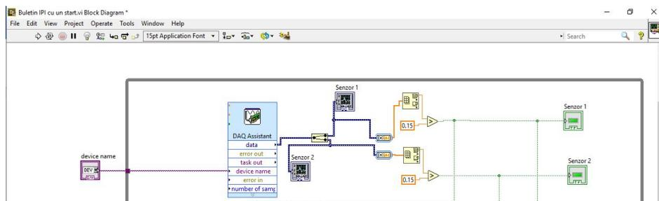
Fig. 5 – The diagram for the acquisition of the analogic signal and its transformation into a digital signal.
