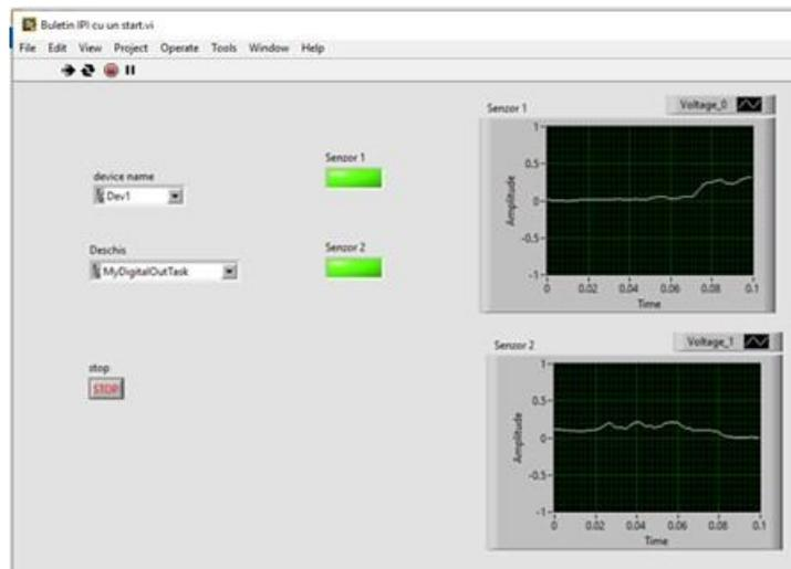
Fig. 4 – The front panel of the virtual instrument for the case „Light off”.
