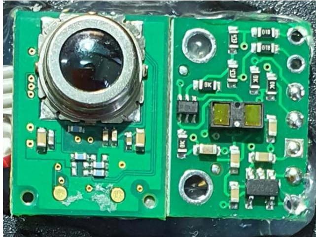
Fig. 3 – Group of sensors (thermal sensor to the left and distance sensor on the right).
