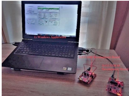
Fig. 6 – Wi-Fi evaluation frame ratio error setup.
