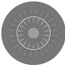
Fig. 4a – Radial perspective of the V1 motor in MotorCad.
