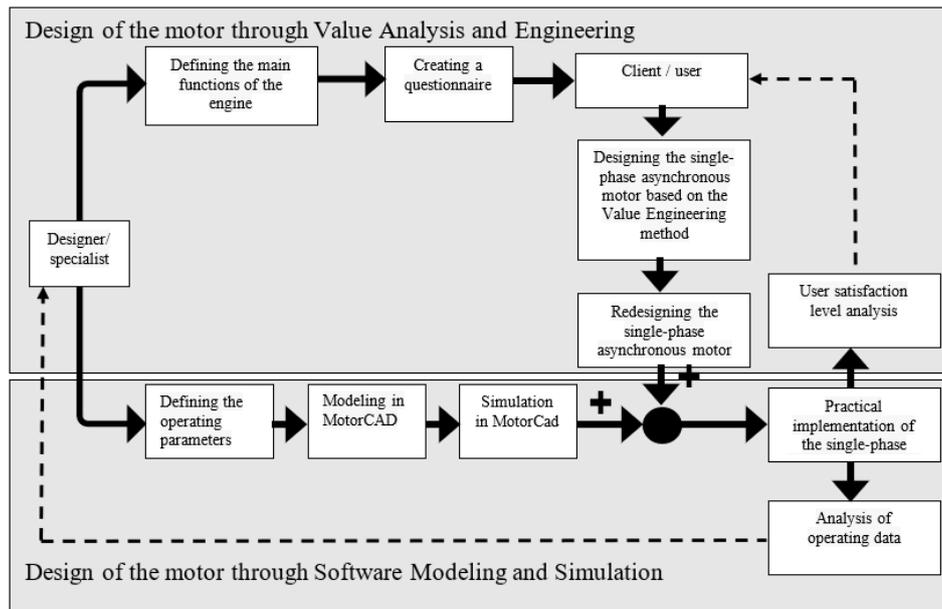
Fig. 1 – Design and redesign stages of a single-phase asynchronous motor.
