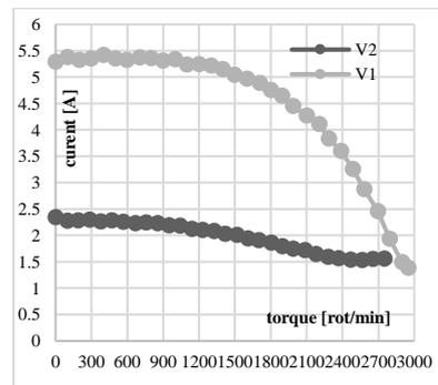
Fig. 9b – Current comparison for the V1 and V2 variants (Lupacescu, 2023).
