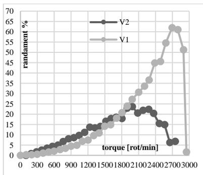
Fig. 9a – Efficiency comparison for the V1 and V2 variants (Lupacescu, 2023).
