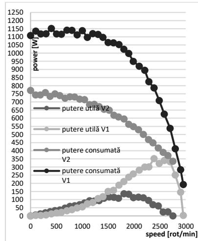
Fig. 8b – Power=f(speed) for the V1 and V2 variants (Lupacescu, 2023).
