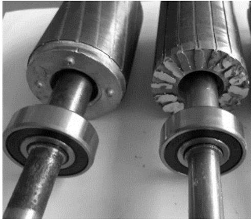
Fig. 7 – Visual comparison between the original rotor (left) and the rotor with rectangular aluminium bars (right) (Lupacescu, 2023).
