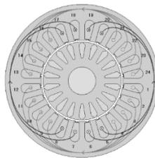
Fig. 4b – Arrangement of windings in slots.
