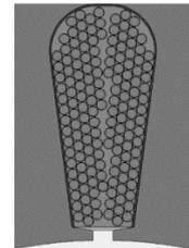
Fig. 4c – Configuration of turns in a slot.
