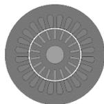
Fig. 5a – Radial perspective of the V2 motor in MotorCad.
