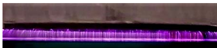
Fig. 2 – Typical discharge by DBD system operating in ambient air.
