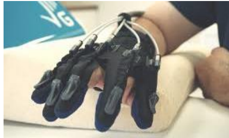
Fig. 2 – Exoskeleton Mechatronic Glove.
