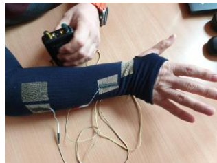
Fig. 6 – Textile Electrodes Glove and MotionStim8.
