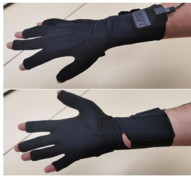
Fig. 3 – Optical-based Sensor Glove (5DT).
