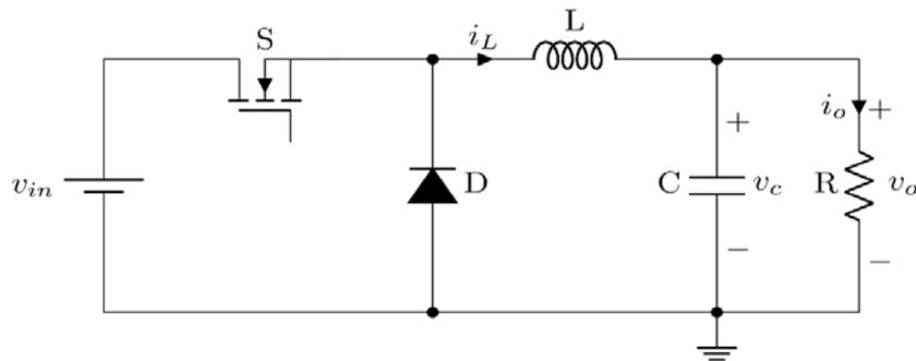
Fig. 1 – Buck Converter.
