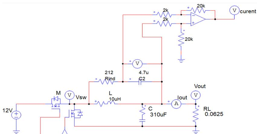
Fig. 4 – Current measurement.
