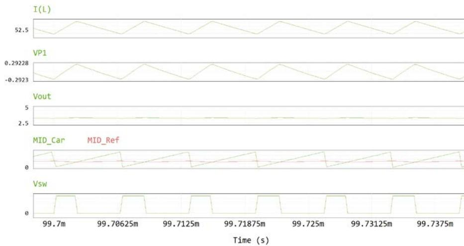
Fig. 9 – Waveforms for the operation of the circuit (from top to bottom): inductor current, sensed voltage proportional to the inductor current, output voltage, PWM carrier and reference waveforms, voltage across diode in the Buck converter.
