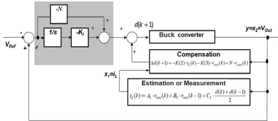
Fig. 2 – PI equivalent form of the state-space controller.
