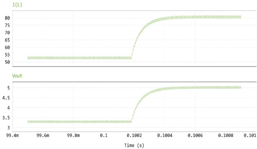
Fig. 8 – Step up change in the output voltage for the simulated circuit.
