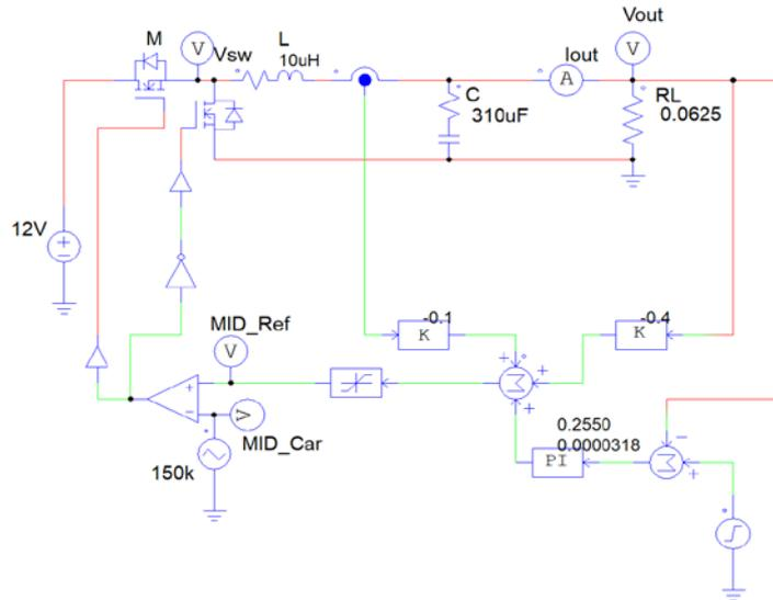
Fig. 3 – Circuit equivalent for the State Space implementation.
